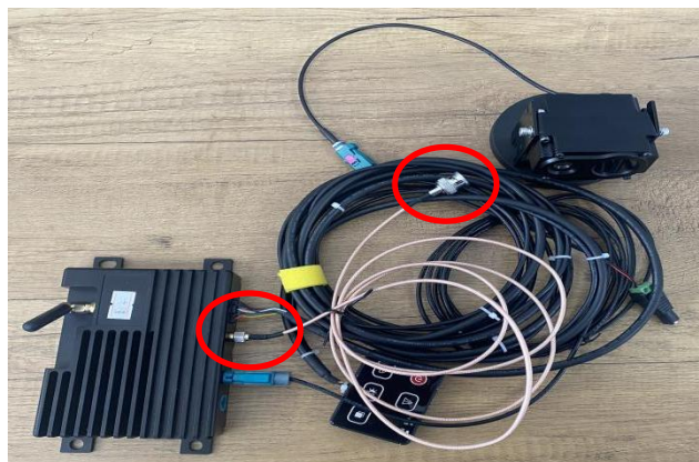
图 15 Connecting the video output cable
