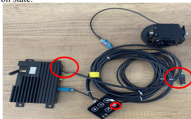
图 16 Connecting the power cable
