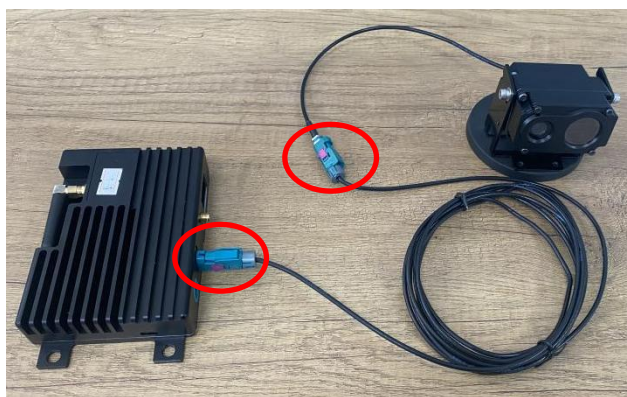
图 14 Connecting the Video Cable
